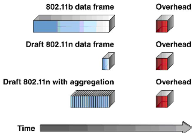
Figure 1: How frame aggregation improves packet efficiencies
