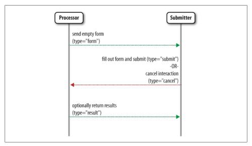
Figure 6-1. Data form interactions follow a simple workflow
