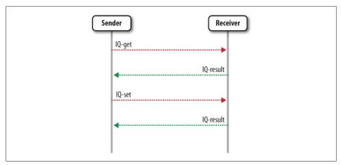
*Figure 2-5.* The IQ stanza provides structured interactions between entities
