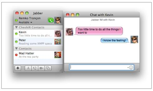
Figure 14-5. Using the CheshiR server component from an XMPP client: CheshiR contacts are mixed with regular XMPP contacts, messages from different contacts get delivered in their own chat dialog, and the message sent to Kevin will result in the message "@kevin I know the feeling!" being posted on Remko's microblog
