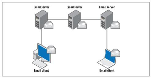
Figure 2-3. The email network has many servers and clients, plus the servers are interconnected in a multi-hop network
