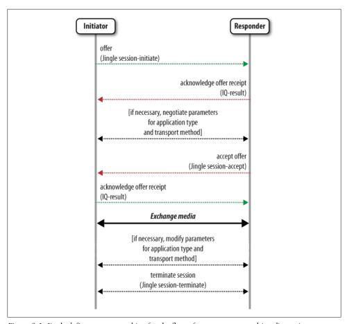
Figure 9-1. Jingle defines a state machine for the flow of a peer-to-peer multimedia session explore these processes later), the responder would eventually send a session-accept to the initiator:
