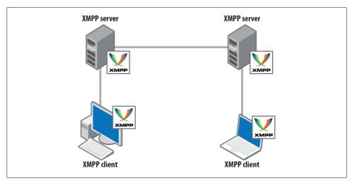
Figure 2-4. The XMPP network has many servers and clients, plus the servers are interconnected in a single-hop network
