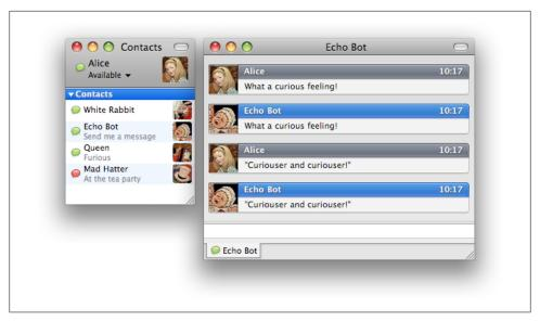
Figure 2-6. The "echo" service in action; "echo bot" acts as an ordinary IM contact, but automatically echoes back every message you send it
